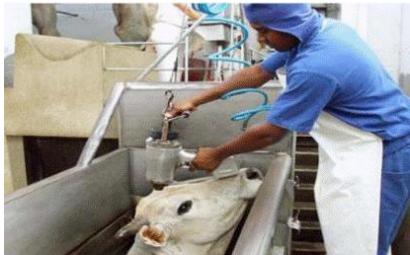
Figure 4.6: Stunner in the correct position
